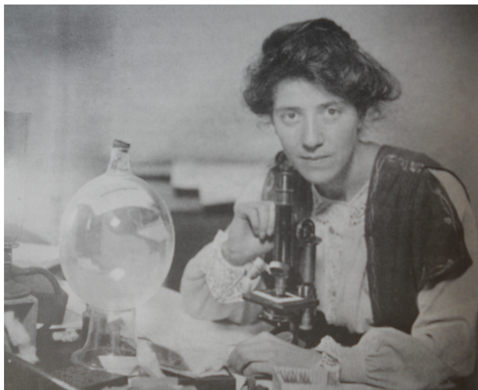
Fig. 1: Marie Charlotte Carmichael Stopes, ca. 1905, perhaps when she was a doctoral student at Munich, Germany. The glass slide on her microscope stage is larger than the usual 5cm x 2cm, but typical of coal-ball sections prepared at that time before the peel technique was applied to permineralized specimens. Her light source is a gas mantle, seen on the left. The spheroidal flask of water may have served to condense this light, but it does not appear to have been used for such a purpose when this photograph was taken (photograph in property of Hugh Person).
